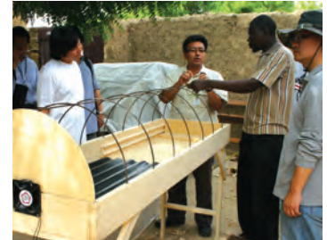
I Hot-wind dryer to produce dried mangoes in Chad
